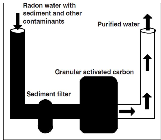
Figure 1: Treatment by activated carbon
